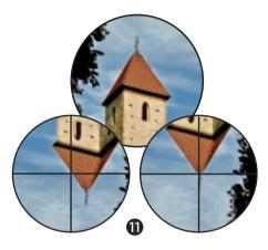
The image reproduced will be upright, but rotated around its vertical axis (you will see a mirror-image). In the finder, however, the reproduced image will be upright and its sides will not be reversed, as above. Now turn one of the two clamp screws (right/left) of the finderscope while looking continuously through the finder. Continue to turn until the finder's crosshairs are exactly over the position that corresponds to what you see when you look through the eyepiece of the main telescope.
