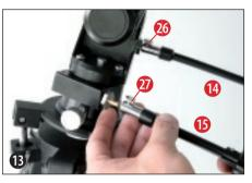
The long flexible shaft (14) (Figure 1) is mounted parallel to the telescope tube. It is secured with a clamp screw (16, 17) on the designated indentation on the shaft.
